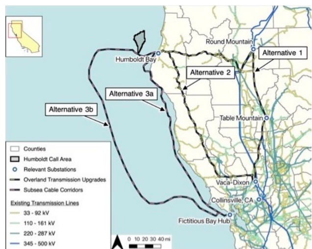
Figure 1. Transmission route alternatives for 1,836 MW wind farm scenario. Source: Schatz Energy Research Center. 2020. California North Coast Offshore Wind Studies Transmission Upgrades Report and Policy Analysis. http://schatzcenter.org/pubs/2020-OSW-R12.pdf .
